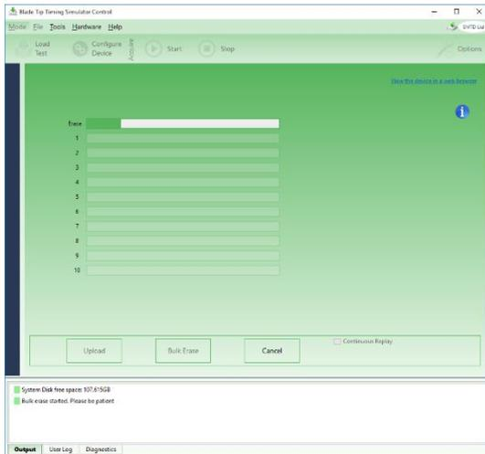
The progress bar indicates how long the process will take and upon completion message appears in the output window with the time to complete. This is typically around 50 seconds. As the device ages this may take longer. If the message fails to appear press the cancel button, recycle the power and repeat the process. Continued failure should be reported back to [enquiries@emtd-measurement.com](mailto:enquiries@emtd-measurement.com)
