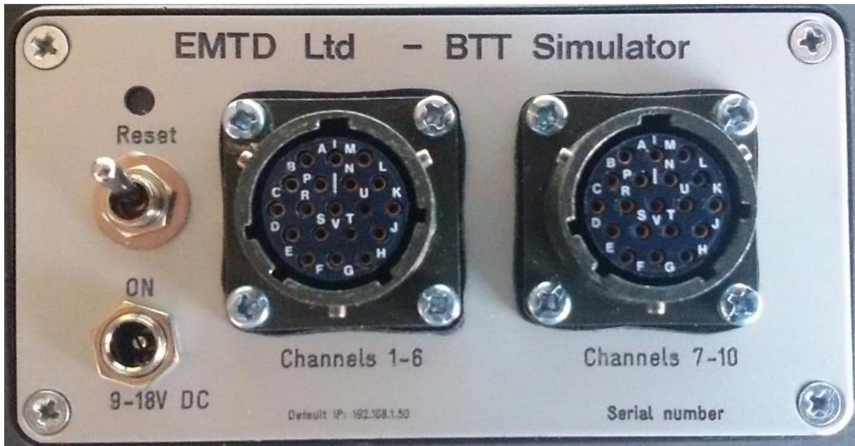
Using a blunt tool to prevent damage to the button gently press and hold the reset button for approximately 5 seconds. On releasing the button the three front panel indicators will flash indicating that a power cycle is required to complete the reset.
