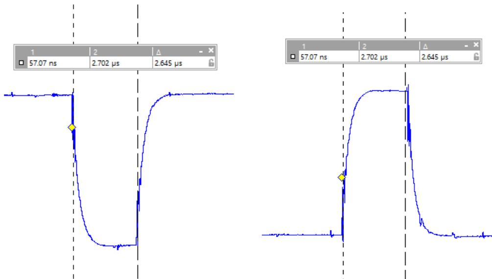
Pulse width is approximately 2.6μS and the rise time approximately 400nS when driving 2m of twisted pair overall screened cable (approx. 200pF cable capacitance). Typical output amplitude when driving 220 Ω. All outputs are AC coupled.
