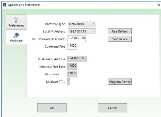
Ensure that the local IP address is correct as the PC may contain multiple LAN connections. Select <sync device> to check the communications with the Simulator.
