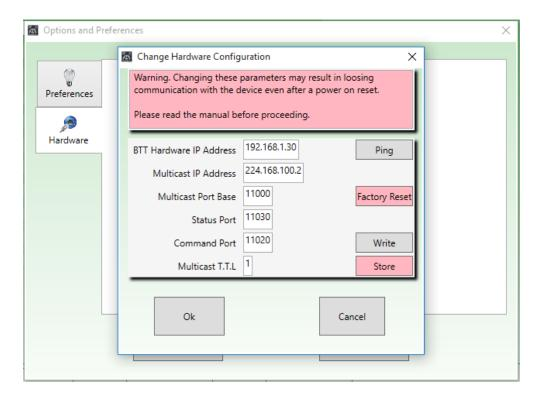
Care should be taken before changing any of these setting as loss of communication may occur. An option to reset to factory settings is available if this problem is encountered.
