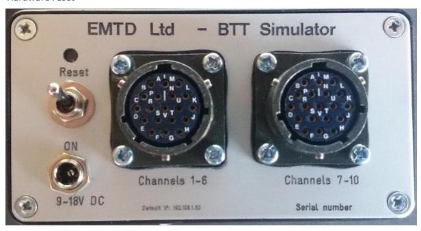
Using a blunt tool to prevent damage to the button gently press and hold the reset button for approximately 5 seconds. On releasing the button the three front panel indicators will flash indicating that a power cycle is required to complete the reset.
