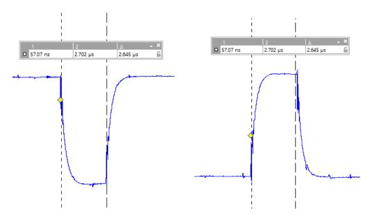
Pulse width is approximately 2.6 $\mu$ S and the rise time approximately 400nS when driving 2m of twisted pair overall screened cable (approx. 200pF cable capacitance). Typical output amplitude when driving 220  $\Omega$ . All outputs are AC coupled.
