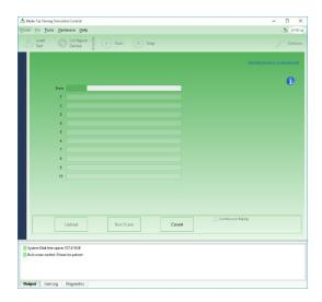
The progress bar indicates how long the process will take and upon completion message appears in the output widow with the time to complete. This is typically around 50 seconds. As the device ages this may take longer. If the message fails to appear press the cancel button, recycle the power and repeat the process. Continued failure should be reported back to <a href="mailto:enquiries@emtd-measurement.com">enquiries@emtd-measurement.com</a>
