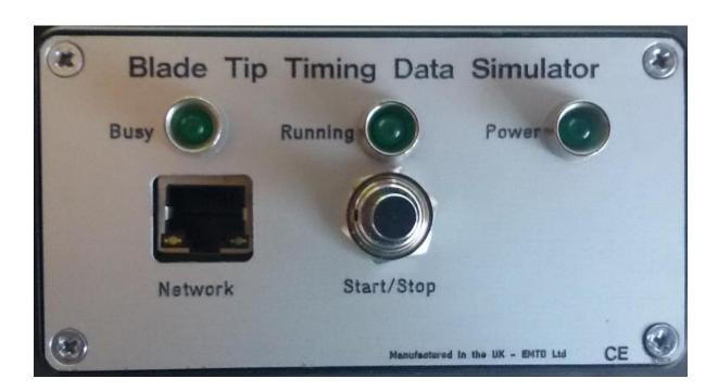
The Simulation can be stopped and restarted at any time by depressing the start/stop button.
