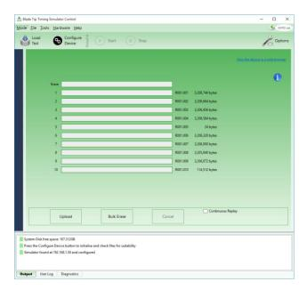
The continuous replay check box is now accessible. Selecting this configures the hardware to automatically restart the simulation after it has completed. Select the Upload button to start the process of transferring data from the PC to the Hardware.
